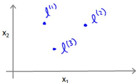
$$\text{例如: } f_1 = \text{similarity}(x, l^{(1)}) = e\left(-\frac{\|x - l^{(1)}\|^2}{2\sigma^2}\right)$$
